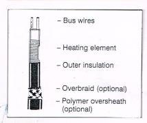
PCS is a parallel circuit constant power cut-to-length tape for use in industrial applications for process maintenance to 140°C.
