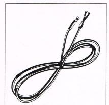
The KDL range of low wattage heating tapes has been developed for the internal and external tracing of drainlines in cold stores, refrigeration rooms and equipment. They are factory fitted with 500mm cold lead terminations. Temperature range: -40°C to 180°C.
